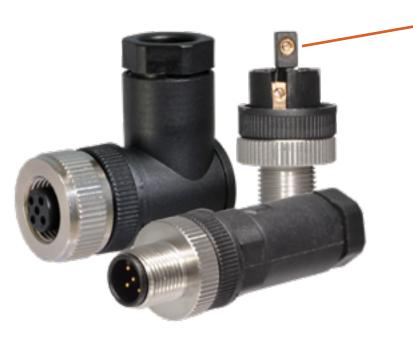
Note the plastic sleeve that covers the centre pin. This is to prevent the bare wires that extrude from the other 4 pins making contact with the copper and creating a short. Not all field fit connectors have this plastic sleeve.
